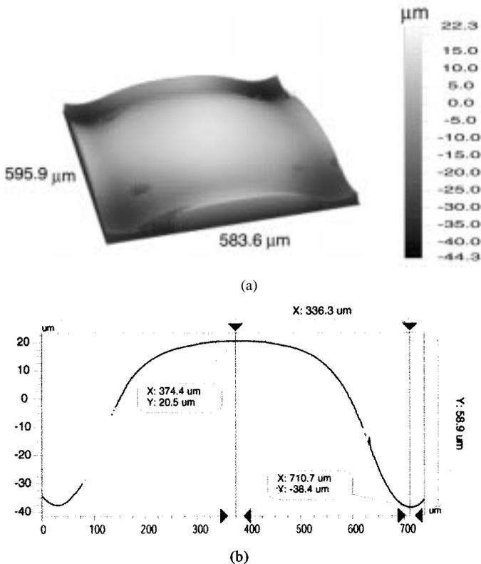
Fig. 9. Segment of a lenslet array patterned in hybrid glass using a grayscale photomask. Each lenslet aperture is a square measuring  $240\ \mu\text{m}$  on a side. (a) Isometric view of the grayscale-patterned surface. (b) Diagonal profile of the surface. Missing data occur due to regions of high slope on the patterned surface.
