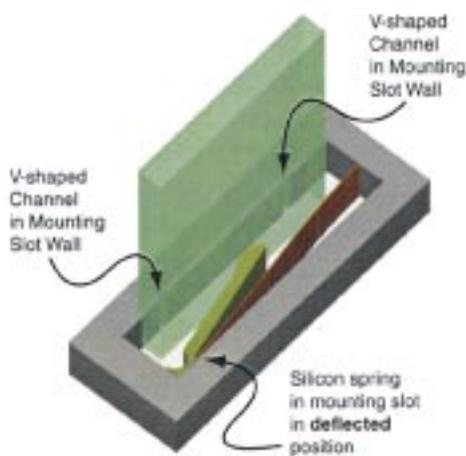
Fig. 4. Assembly of optical elements and MOT substrate.
