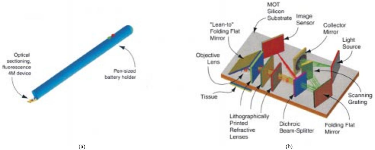
Fig. 1. Pen-sized miniature microscope. (a) A conceptual, scaled diagram of a pen-sized imaging probe equipped at the tip with a multi-modal miniature microscope (4M). (b) A magnified view of the 4M-device layout. The 4M device measures 9 mm in length, 5 mm in width, and 3 mm in height.
