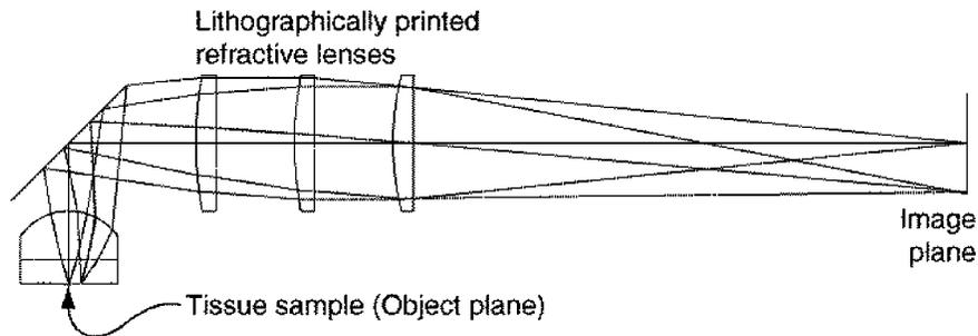
Fig. 2. Optical design of a miniature microscope objective. The figure shows the design form of an  $NA = 0.4$ ,  $m = -4$  microscope objective with a field of view of  $300 \mu\text{m}$ . This is the microscope objective used in the complete 4M device shown in Fig. 1.
