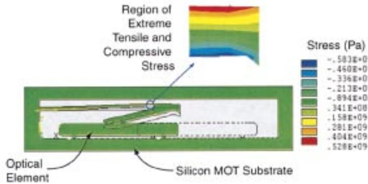
Fig. 3. Silicon-spring displacement and the normal stress in the horizontal direction. The optical element is shown in its penultimate position. The highest tensile stress (shown in red) is predicted to occur at the top of the spring in this diagram. The predicted maximum tensile stress in the silicon spring is less than the failure stress of silicon, thus validating the design of the silicon spring. The thickness of the optical element is  $150\ \mu\text{m}$ .
