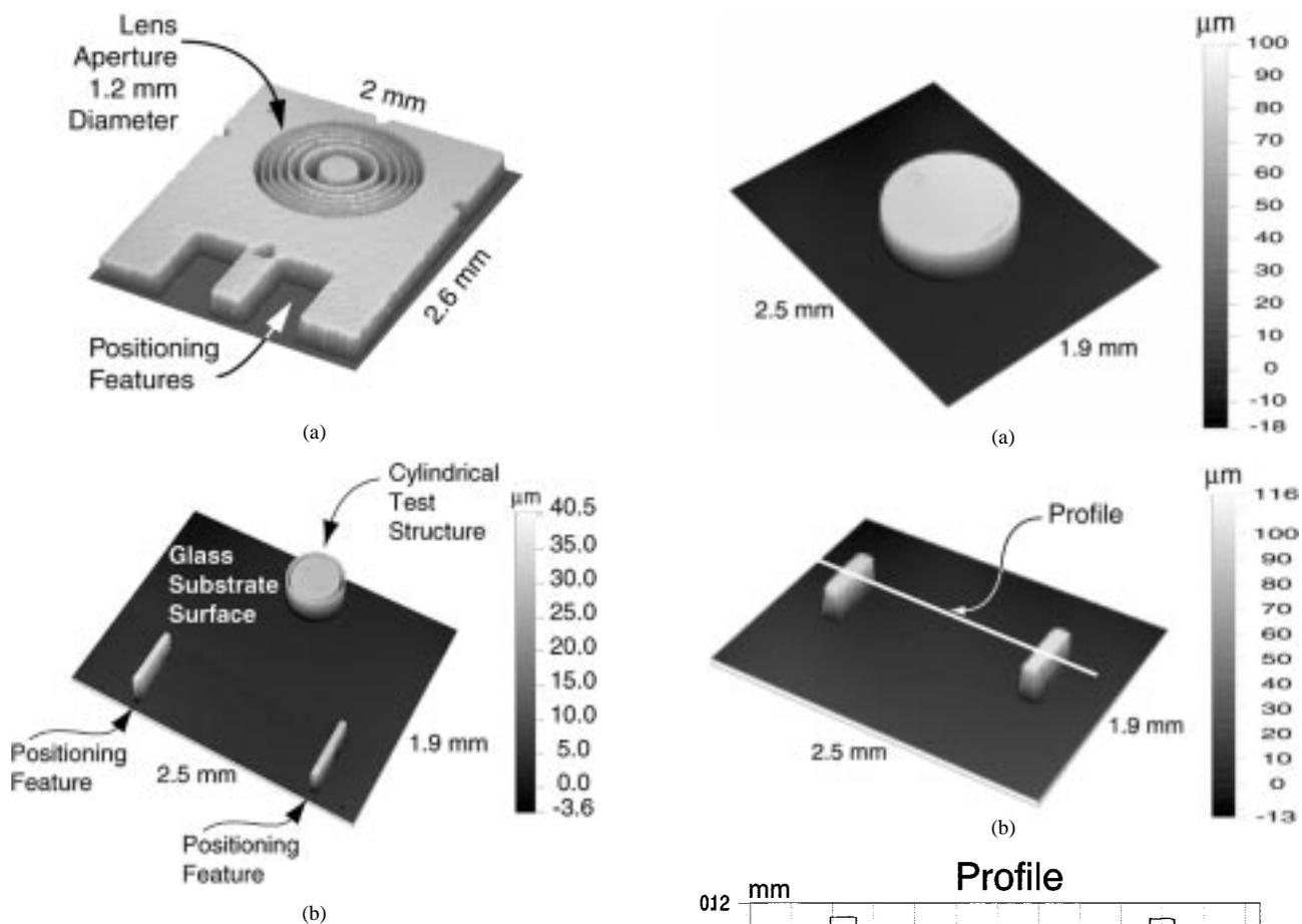
Fig. 7. Lithographically patterned optical elements. (a) A microoptical element patterned in hybrid glass material on a  $150\text{-}\mu\text{m}$ -thick glass substrate. The thickness of the hybrid material is  $17.8\text{ }\mu\text{m}$ . The positioning features are of an earlier, recessed design [11]. (b) A more recent test element made with hybrid glass material patterned to a depth of  $34\text{ }\mu\text{m}$ . The positioning features now protrude from the substrate.
