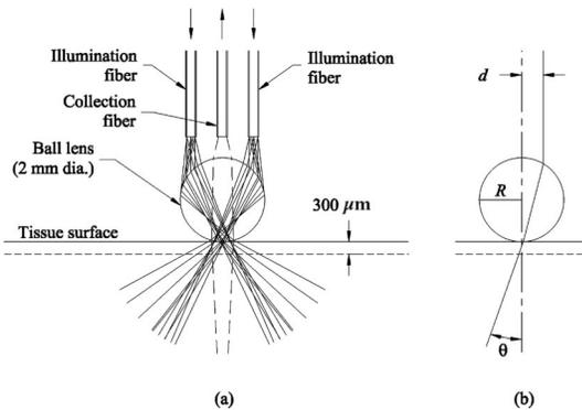
Fig. 1. (a) Ball lens coupled probe, showing illumination ray paths (solid lines) and collection region (dashed lines). A typical epithelial thickness of  $300\ \mu\text{m}$  is shown for reference. (b) Angular deviation of a ray incident parallel to the probe axis.
