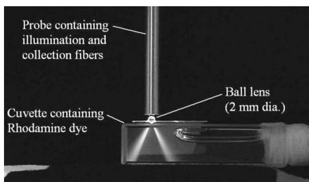
Fig. 2. Photograph of the ball lens coupled probe illuminating a cuvette containing the fluorescent dye Rhodamine.
