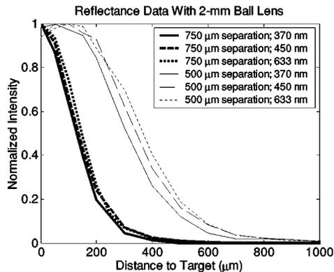
Fig. 3. Normalized reflectance signal as a function of probe-to-target distance. Source–detector separation and illumination wavelength are noted. Half-maximum intensity occurs at an average distance of 136  $\mu\text{m}$  (for 750- $\mu\text{m}$  separation) or 340  $\mu\text{m}$  (for 500- $\mu\text{m}$  separation).
