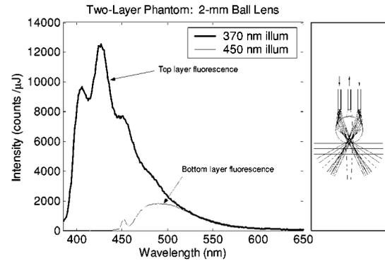
Fig. 5. Two-layer tissue phantom fluorescence data: ball lens coupled probe with a 2-mm-diameter ball lens and 750- $\mu\text{m}$  source–detector separation, corrected for excitation energy.
