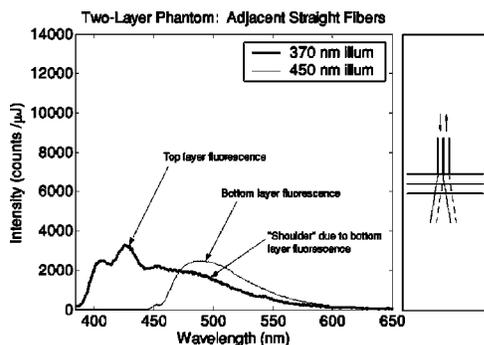
Fig. 4. Two-layer tissue phantom fluorescence data: straight fiber probe at a minimum source–detector separation (250  $\mu\text{m}$ ), corrected for excitation energy.
